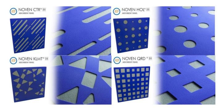
NOVEN® is a perforated flat shape acoustic panel. It is made of flexible open-cell acoustic foam with a rigid housing of perforated ABS, with coloured velvety finishing. This attractive product allows the combination of two colours; the colour of the housing and colour of the fabric colour, giving its appearance several appealing colour combinations. The inner absorbing core is made of open-cell acoustic foam composing the inner absorption core with fire-resistant fabric finishing.
